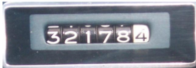
The odometer pictured has six digits—“columns” of spinners labeled 0–9. Now imagine there are only two columns of spinner labeled 0–1. At what value do we stop?
