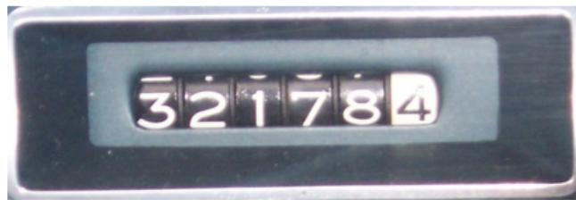
The odometer pictured has six digits—"columns" of spinners labeled 0–9.
