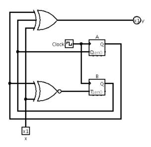
*Note:* The "A" flip-flop (on the top of the diagram) is a D flip-flop, while the "B" flip-flop (on the bottom) is a T flip-flop.
